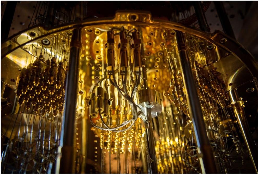
The Quantum Systems Accelerator will optimize a wide range of advanced qubit technologies available today. Berkeley Lab uses sophisticated dilution refrigerators to cool and operate superconducting quantum processor circuits. (Credit: Thor Swift/Berkeley Lab)
